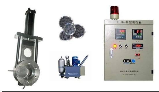
This DHB series of screen changer consists of main body, slide plate, heater and hydraulic unit with accumulator. It is driven by hydraulic power, and the slide plate carries 2 pieces breaker plates can move linearly in both directions to achieve screen changing in a short time.
